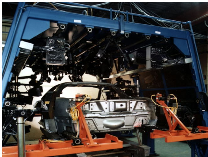
Figure 1. In-line machine vision system measuring a car body.
