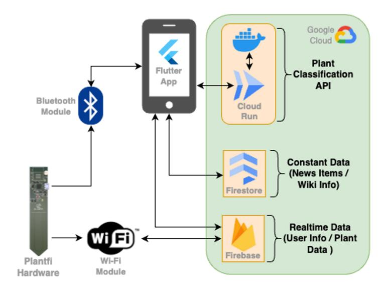
The software architecture incorporates on-device and cloud-based solutions to enable our objectives.
