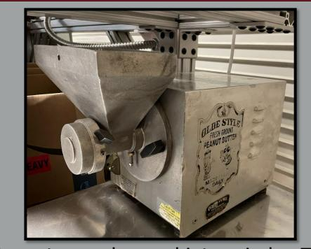
Peanuts are dropped into grinder. The grinder grinds them into peanut butter and deposits the peanut butter into a container
