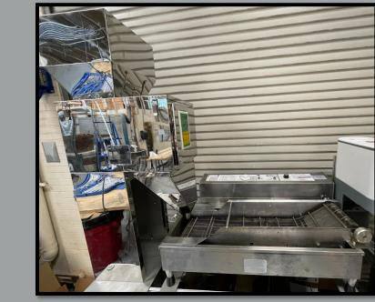
Peanut dispenser drops peanuts into a retrofitted Belshaw Donut Fryer. The fryer's automated conveyor moves peanuts through oil
