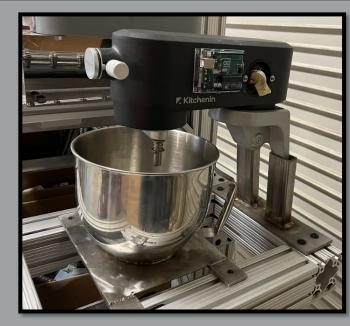
A retrofitted stand mixer is activated when peanuts & seasoning enter. A trap door on the bottom of the bowl opens & peanuts exit
